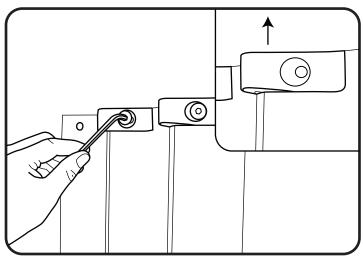
Remove the screws from the Upper Clips on the damaged Uprights using a 5mm allen key. Remove these Upper Clips by sliding upwards.
