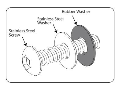
Assemble the fixings as shown above. Have one person hold the sign in position and align the fixing points. Insert the screw and washers and tighten well using the allen key provided.
