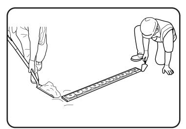
Using a quick setting concrete fill around the socket and smooth for a neat finish. Again, ensure socket is level. Clean any debris from the top of the socket.
