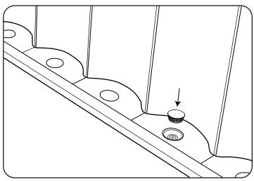
Position the screw covers over the tightened screws and secure into place using a rubber hammer.
