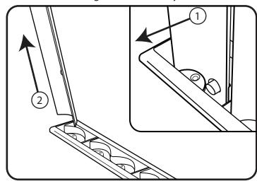
Tilt back Upright and lift out of socket.
