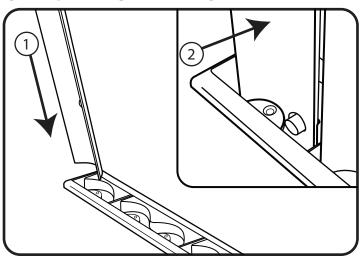
Lay out all the uprights on the ground in order then begin inserting the upright into the sockets at a slight angle and push forward to locate hole in upright onto the pin in socket.
