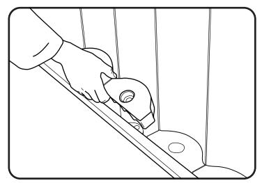
Insert socket covers by hand and use a rubber hammer to secure into place.
