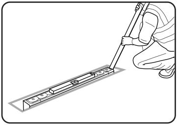
Ensure socket is level, add/remove gravel as required.
