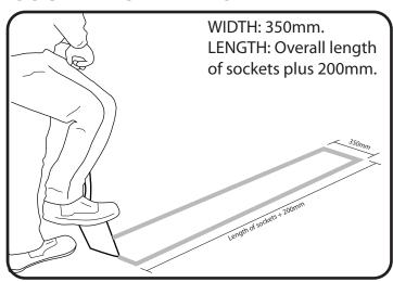
Measure the size of the hole to be excavated. Check for buried services then dig the hole to a depth of 450mm. Line the hole with 50mm of gravel for drainage and ensure base of hole is flat.
