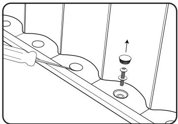
Remove the Screw Covers from behind the damaged uprights. To do this use a flat head screw driver or similar to prise the covers off. Remove the screws from beneath using a 6mm allen key.
