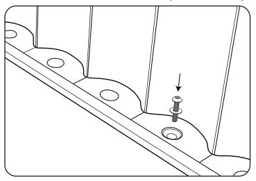
Fix the socket covers to the socket using the M10 screws and washers provided. Tighten using the 6mm allen key provided or use a hand drill if available.
