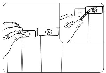
Secure clips using the M8 countersunk screws and tighten using the 5mm allen key provided. For speed use a hand drill if available.
