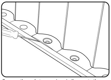
Remove the socket covers in a similar way to the removal of the screw covers.
