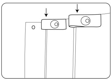
Each Upper Clip is located between two Uprights. To attach slide the Clip down onto the Uprights.
